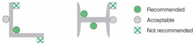
Fig.4: Recommendation to install cables in steel beams
