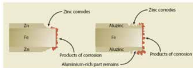
Edge corrosion of hot-dip galvanized steel (left) and of Aluzinc (right).
