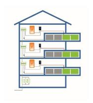
Balcony system consisting of plug-in modules with micro inverters (grey) and standard modules for water heating (green).
